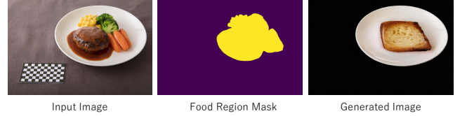
Figure 3: Inpainting result using the default Stable Diffusion v2 model. The model hallucinates food, which motivated our fine-tuning approach.
