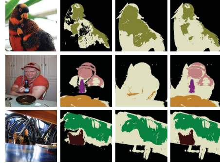
Figure 2. (1)input image, (2)estimated mask by single-class model, (3)estimated mask by multi-class model, (4)integrated mask
