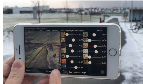
Figure 1: The world’s first real-time multi-style-mixing transfer app, “DeepStyleCam”, running in about 5 fps on an iPhone 7 Plus. See the demo video in the supplementary material. This app is available on the iOS App Store. Please search for “DeepStyleCam”.
