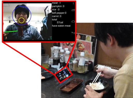
Fig. 1. A typical usage of the proposed system. A smartphone on which the proposed system is running is put toward a user’s face. It continuously detects eating action and estimates food categories of eaten foods.
